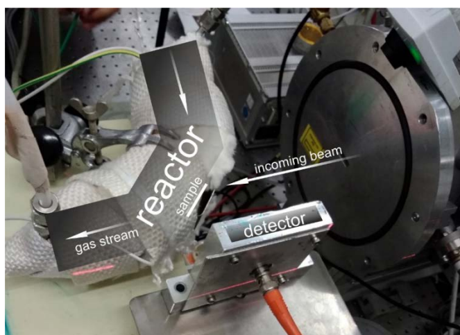
Fig. 2: experimental setup of the self-designed XAS reactor for in-situ measurements at beamline P65, DESY, Hamburg.
